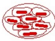
A *flocculated* structure assumes a random tip to side orientation much like a "house of cards" whereas a dispersed structure has the platelets more or less aligned to
